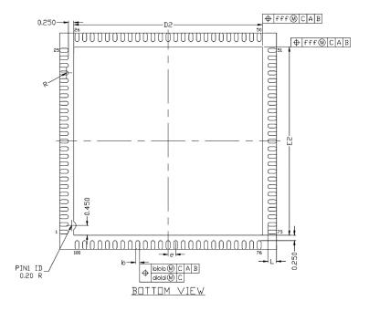
Figure 3 Package Outline Drawing of QFN100 10x10mm<sup>2</sup>
