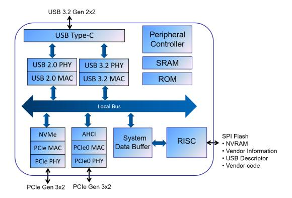
Figure 1 Block Diagram - JMS586A
